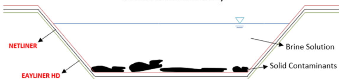
Double liner system / Leak detection layer for toxic or hazardous leach solutions
